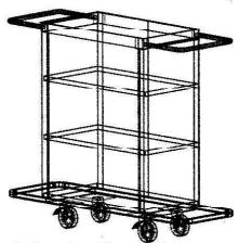
6, 2 handrails and upper tray are fixed on the side boards with screws.
